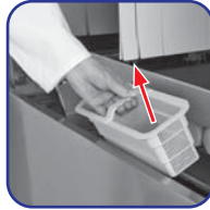
Remove and wash strainer baskets
