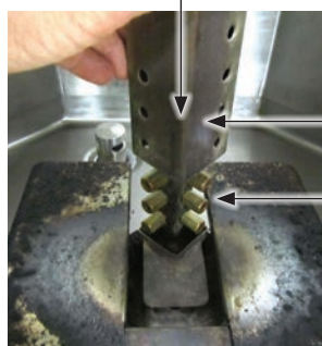
Install Flame post guard over Flame post
