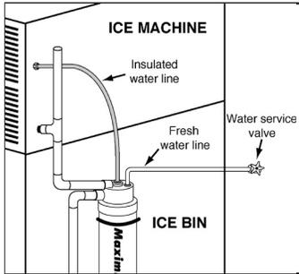
Insert the tubing containing the fresh water source into the outer fitting (connection #1) on the top of the Maximicer unit. If additional tubing is required between the Maximicer and the wall outlet or water filter, connect additional tubing to existing tubing with a compression union.
