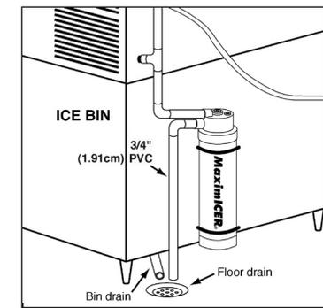
Connect a PVC line to the lower PVC connection on the Maximicer using a 90° fitting (connection #4). Plumb a vertical line down then run horizontal to the floor drain.
