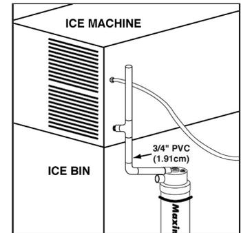
**WARNING: Water will overflow into the ice bin if the PVC line is installed horizontally after exiting the ice machine.**
