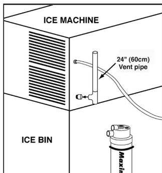
5 Plumb PVC line from ice machine to Maximicer.
