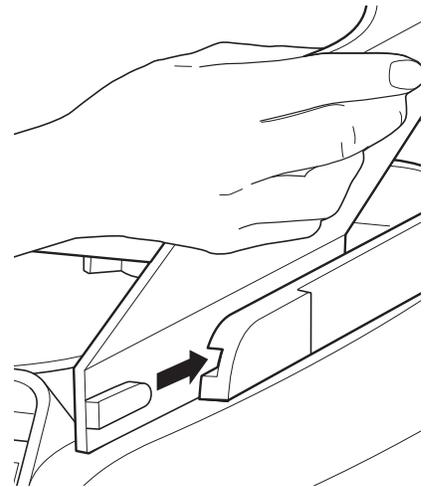
Slide Quiet Shield™ into place. If necessary, hold the edges of the shield open to ensure a secure fit.
