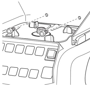
Install thumbscrews to secure Quiet Shield™ to upper base housing.
