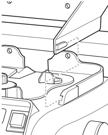
Align the dovetail joints along the base of the Quiet Shield™ with the cutout notches on the upper base housing.
