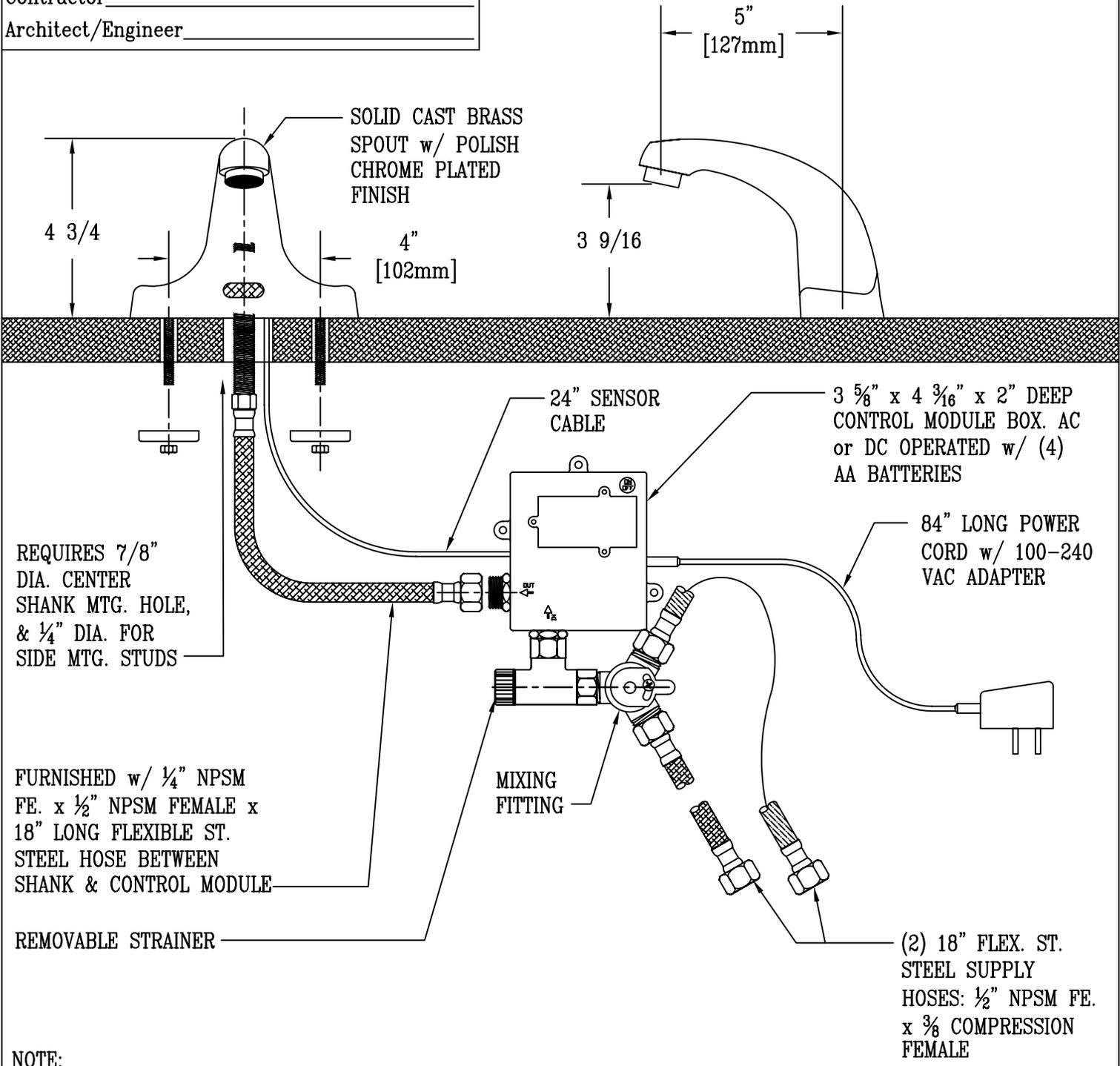
REQUIRES 7/8" DIA. CENTER SHANK MTG. HOLE, & 1/4" DIA. FOR SIDE MTG. STUDS
