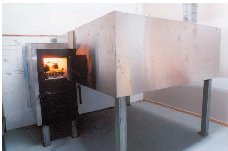
This oven has the fire box on the side. This is optional
