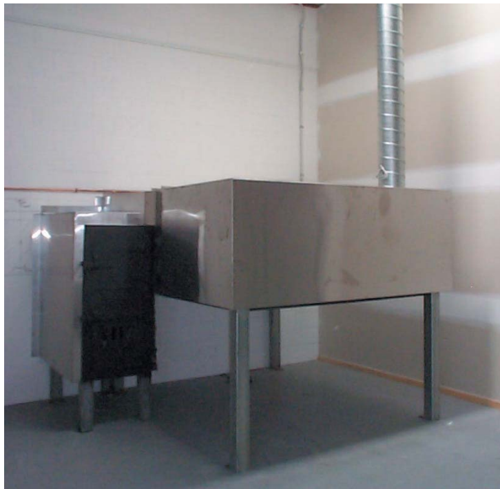
Oven is covered in architectural finish in this case Stainless Steel
